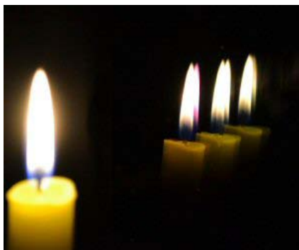
Triple glazing with LE coating of outside of the innermost pane. Indicated by red color of the second of the six reflexions
