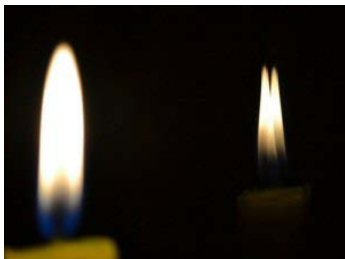
Single glass reflection. You can clearly see the reflexions of both sides of the single pane of glass
